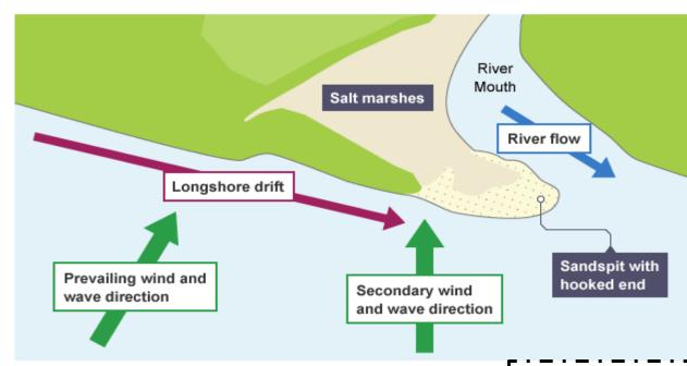
The diagram shows the building of a spit by longshore drift across the mouth of a river.
